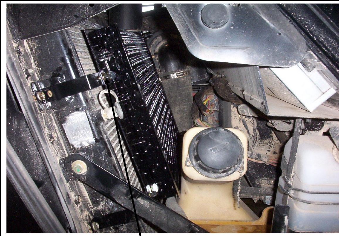
Use the wing bolts to secure the right end of the condenser coil to its mount brackets.
