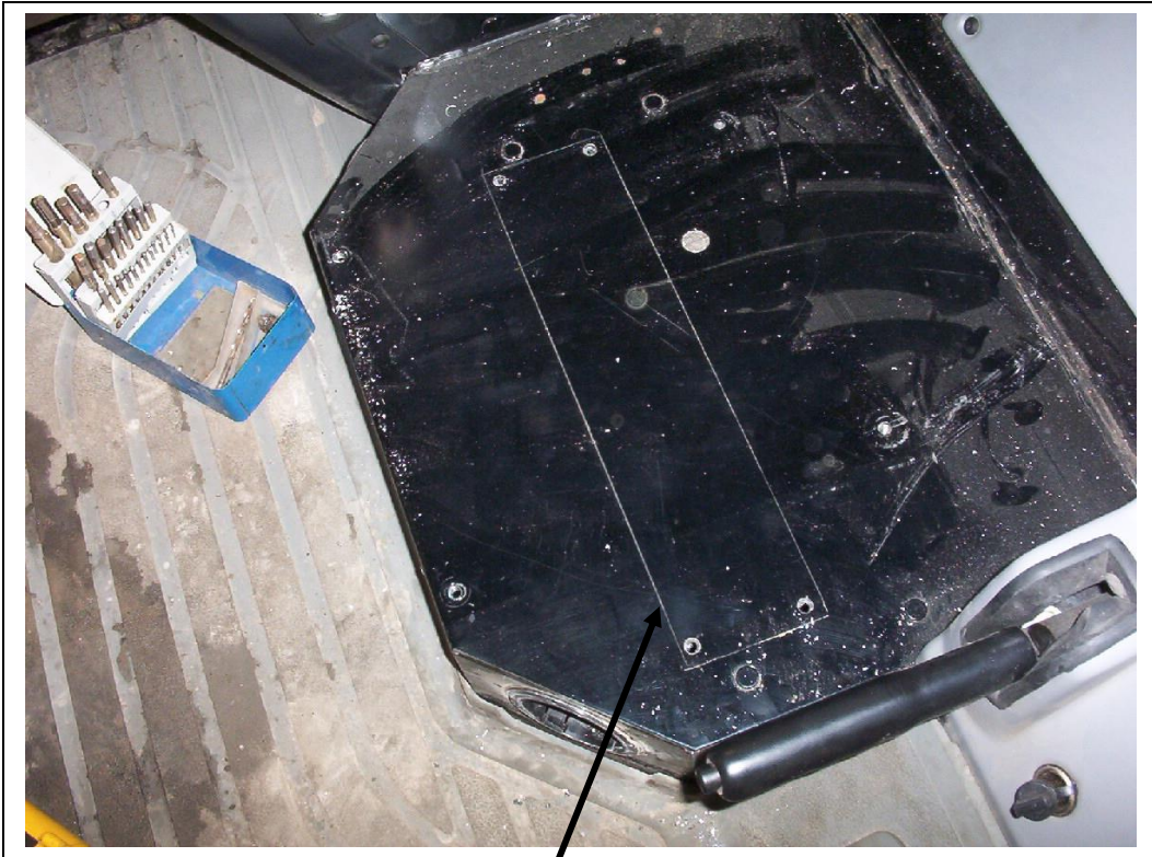
Hole scribed and pilot holes drilled for jigsaw blade.
