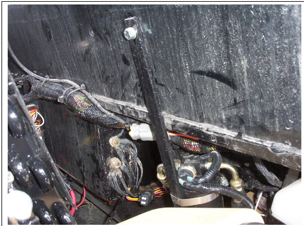
Drier mounts to forward side of mount bracket.
