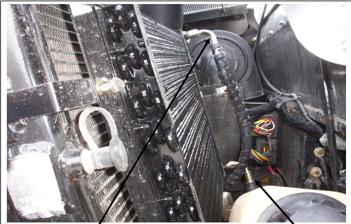
13/32" hose on condenser
