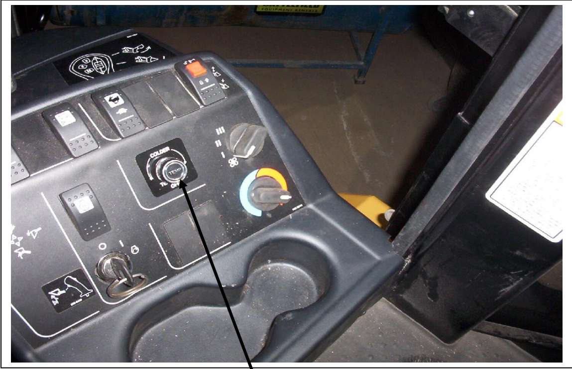
Thermostat and decal in place in right hand control console.
