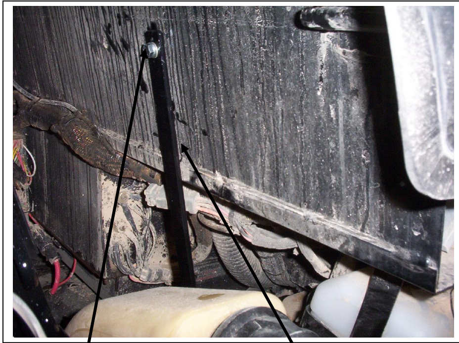
M8 x 25mm bolt, lock and flat in threaded hole.
