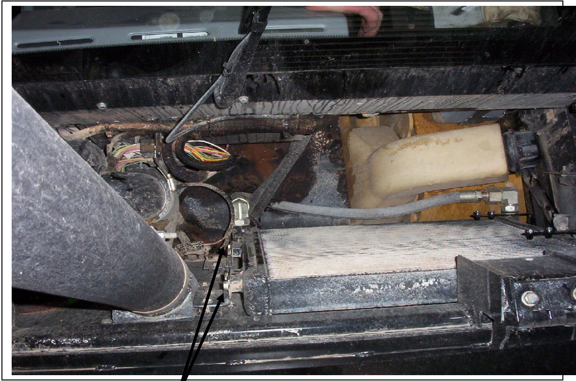
Loosen the inside set of bolts on the left end of the oil cooler.
