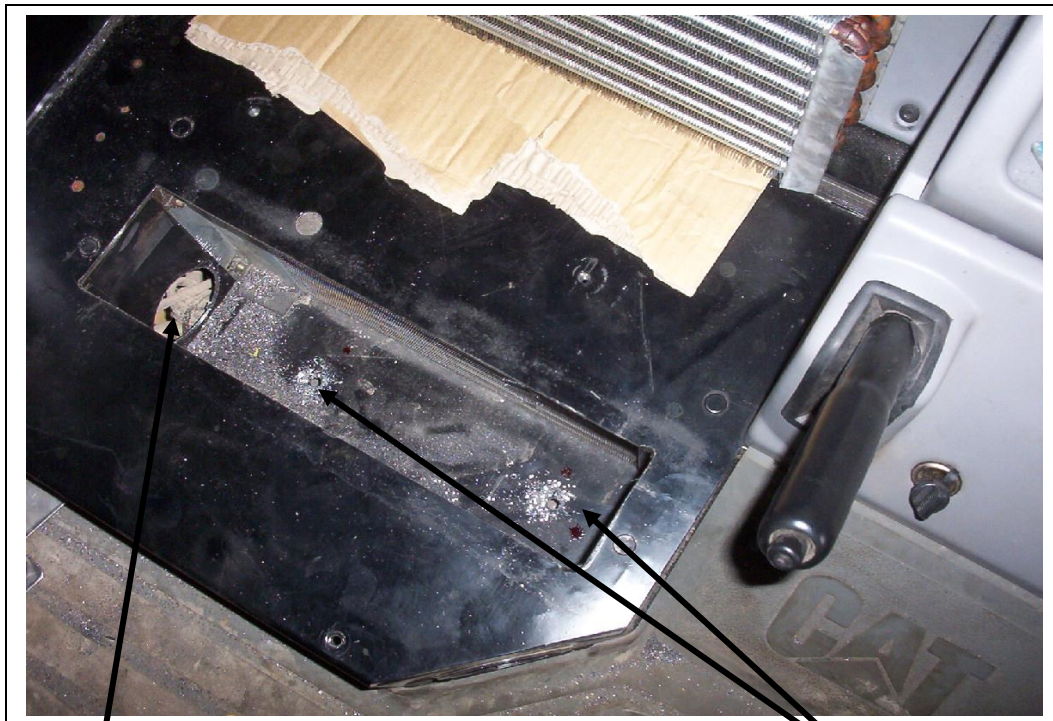
Hole scribed and pilot holes drilled for jigsaw blade.
